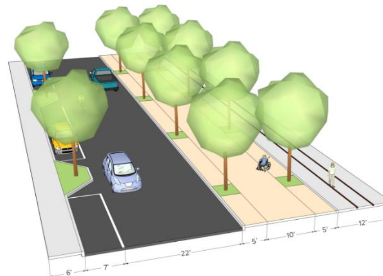
Figure 6-2: Planned Street Section of Pennington Avenue
