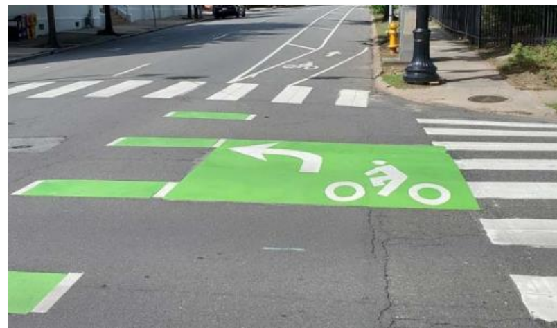
Figure F-25: Two-Stage Turn Queue Box Marking
