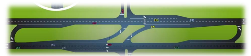
Figure F-4: Reduced Left-Turn Conflict Intersection Plan
